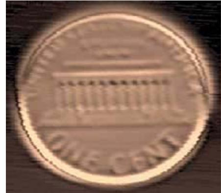
Photo 1. This image is produced not by light but by scanning it with an eddy current probe containing an SDT sensor. The pixel resolution is 0.1 mm on both axes. When you monitor the perturbations in eddy currents caused by surface irregularities, the probe behaves as a differential proximity sensor. By measuring the magnitude of the signal, you can obtain information about the coin material.
